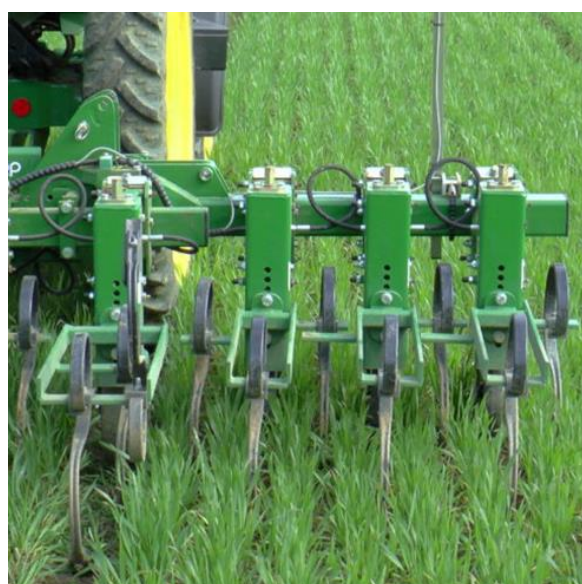
“Robocrop” inter-row cultivator, guided by robotic ‘eye’.
