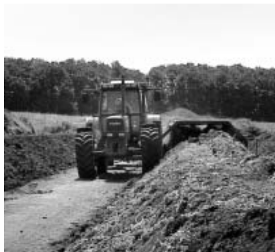
Aerobic windrow composting is the most popular composting method, and involves maintaining oxygen in the pile by regular turning
