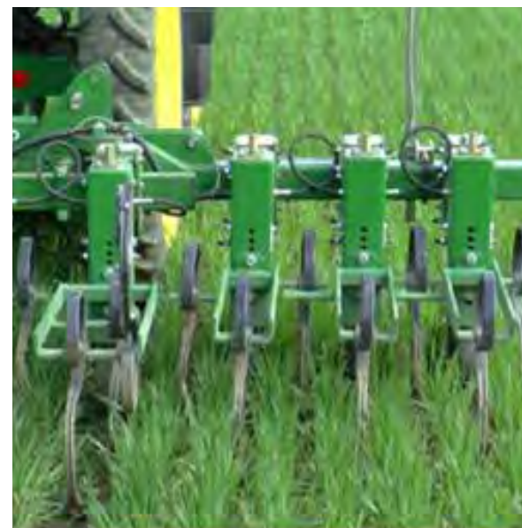
'Combcut'. Manufactured by LyckeGard. The Combcut provides a post-emergent check on weed growth, invented by a farmer who recognised the potential to exploit the physical difference between young cereals (monocots) and the broad-leaved weeds (dicots) with their stronger stems.
